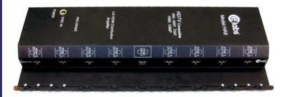
Integrated HCRS (HDMI Cable Retention System). Prevents accidental disconnects and service calls.
